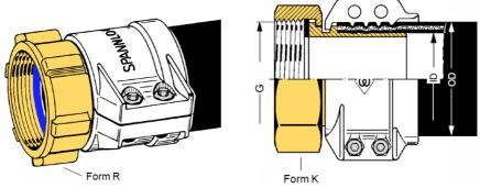
Female hose fittings with re-usable Spannloc bolted clamps of hot stamped aluminium. Bolts and nuts steel zinc plated and chromed. Working pressure up to 25 bar. Chemical resistance chart see page 250.
