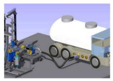
The Master Meter consists of a standard series P.D. Meter (mounted in a Carry Frame, mobile trolley, Road Going Trailer or Skid Base). The direction of flow through the meter is indicated by arrows on the meter manifold. It must be emphasized that the Master Meter, although robust, is a precision instrument and must be properly handled and treated to ensure that it maintains its accuracy.
