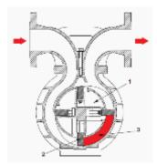
The product enters the measuring chamber following the direction of the arrow. The rotor and blades assembly (1-2) is set in motion by the pressure of the liquid on blades. A certain amount of liquid (3) is held between 2 blades and then directed to the discharge manifold. The volume of liquid measured at each rotation is therefore equal to 4 times the measured quantity (3). The smooth curves the meter pieces provide a steady, non-fluctuating flow resulting in low head loss.
