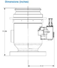
The Model 352GF Hydrant Pit Valve is a Deadman operated on/off valve designed for use in aircraft refuelling. It typically bolts to the terminus of an underground fuel delivery piping system and qualifies as the final shut-off device for such systems per NFPA 30.
